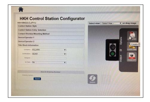
Below is the pdf drawing generated from your design with an exclusive drawing number that will be a permanent identification to the control station you created. The "HKHMODxxxxxx" part number is assigned to this design. If changes need to be made to this design, a new model must be created that will generate another exclusive drawing number.
