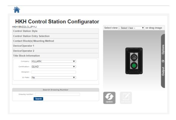
In this case the designer noticed they forgot to include a hub, so before clicking onto the Output Options bar, go back to the drop down options and click on the drop down for Control Station Entry Selection and choose a hub requirement. Click on "Update" again to refresh the view and review your changes.
